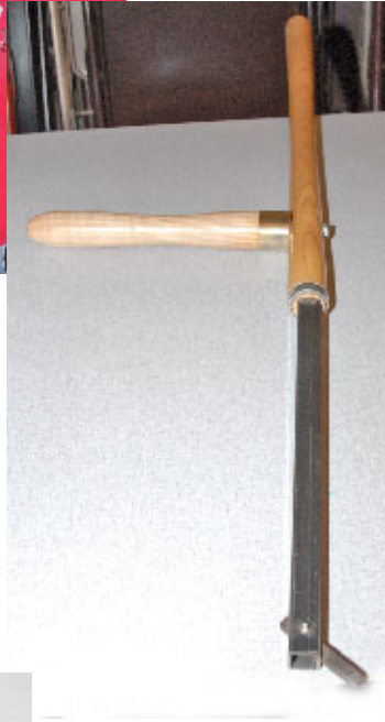
Jim Oates presented a hollow vessel turning tool from square tube with ash handle from a shovel and a shallow leaf-carved maple bowl.
